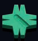
Application: Simply run the tool down the positive side of the Wera magnetiser/demagnetiser and the tool immediately becomes magnetised and is able to hold the screw securely on the blade. To demagnetise the tool, simply run it down one of the four negative sides.
