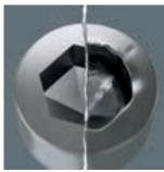
Hexagon screws can endure a problem because the contact surfaces delivering the power from the conventional tool, is transferred to the screw via very small surface areas. The consequence: the screw can become damaged (rounding out). Hex-Plus tools have a greater contact surface that
