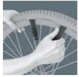
With the glass fibre reinforced plastic tyre jacks, the tyres can be safely levered off the rim without damaging the rim. Lift off of the rim with one tyre jack, hook into a spoke and pull off the tyre with the second tyre jack. The two tyre jacks can be clicked together and are therefore not lost individually.
