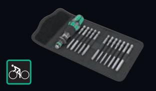
13-piece set, in a pouch; 1 816 R Kraftform bit-holding screwdriver handle with Rapidaptor quick-release chuck, suitable for  $^{1}/_{4}$ " hex bits as per DIN ISO 1173-C 6.3 and E 6.3 and Wera series 1 and 4; 12 bits, 89 mm long, tough, for universal use
