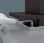
All users will recognise the need to saw or grind down L-keys to make them shorter for particularly confined screwdriving jobs. This has the disadvantage that they no longer have any corrosion protection at the separation point and secondly, they can become "soft" and therefore useless due to an
