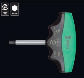
Application:Hexagon socket screwsPre-set torque:4,0 Nm, 5,0 Nm; fixed pre-setAccuracy:±10 %. Reliable slipping mechanism and acoustic signal<br/>when reaching the set torque.Blade:RoundDesign:Hex-Plus, brushed chrome-plated finish, Black PointHandle:T-handle, multi-component
