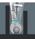
The Joker 6003 combination wrench with its special mouth geometry – an open-end offset by 7.5° and the double hexagon profile – doubles the placement possibilities when repeatedly turning the wrench 180° around the longitudinal axis. Bolts and screw heads can be "accessed" every 15°. The
